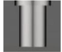
» **Recommended Hole Depth** - Allows for proper insert set down (flush to 0.005 inch below the surface), prevents excessive flash, and prevents back filling of plastic from entering bottom threads.
